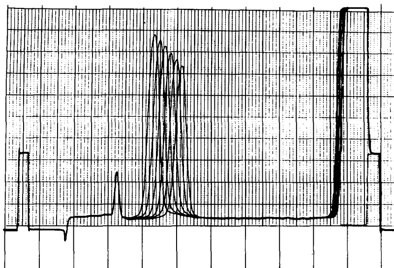
Fig. 4. Schlieren sedimentation velocity boundaries of unfractionated citrus pectin. MSE Centriscan 75; monochromator setting = 546 nm; rotor speed = 44 000 rev min -1 , temperature = 20°C; scan interval = 28 min; loading concentration = 6.0 mg ml -1 . Direction of sedimentation is from left to right.
